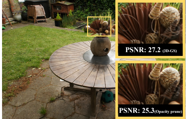
Figure 3. Zero-shot Opacity-based Pruning. A significant number of Gaussians exhibit small opacity values (top). Simply utilizing Gaussian opacity as an indicator for pruning the least important Gaussians results in the rendered image losing intricate details (bottom), with the PSNR dropping from 27.2 to 25.3. This has inspired us to find better criteria to measure global significance in terms of rendering quality.
